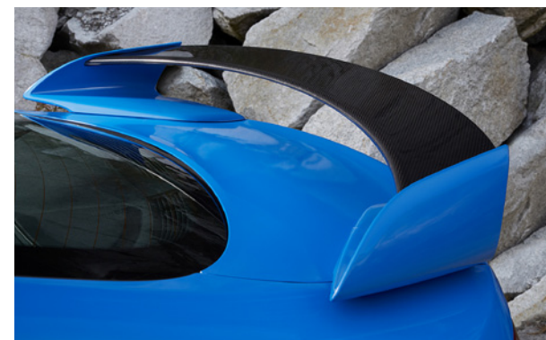
Bootlid spoiler and other bodywork revisions reduce lift by 68%
